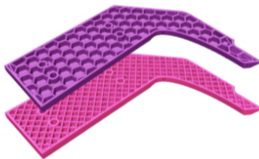
Figure 3.7: Hexagonal (top) compared to rectangular (bottom) infill pattern
