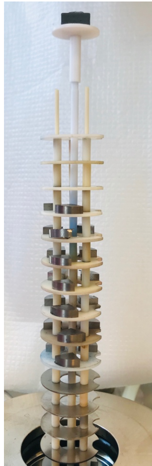
Figure 6.6: Illustration of titanium pieces placed in the TG machine
