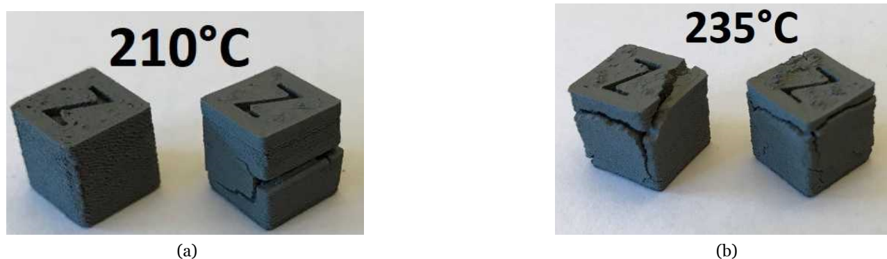
Figure 6.3: Illustration of the sample cubes which were printed at 210°C (a) and 235°C (b) respectively
