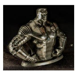
While prints made with Filamet<sup>™</sup> can be polished to a beautiful shine in their green state, many applications dictate post-processing. Filamet<sup>™</sup> again surpasses other metal AM solutions by debinding with simple heat – no catalysts, no solvents, no safety risk.
