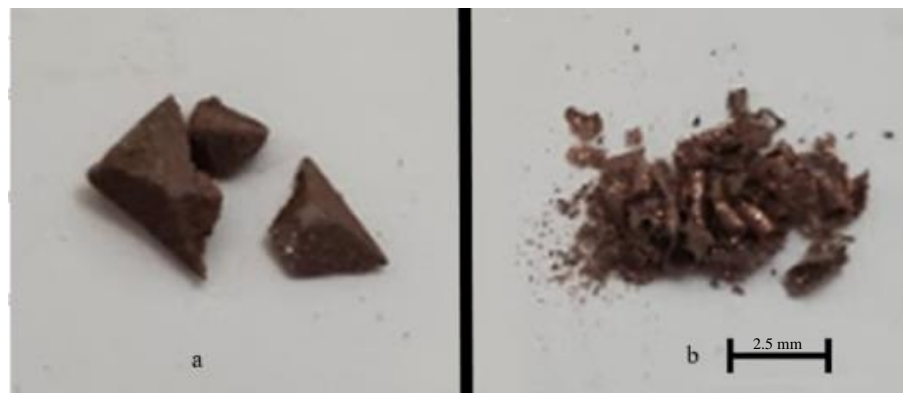
Figure 10: TGA test samples (a) filament pieces (b) filament powder
