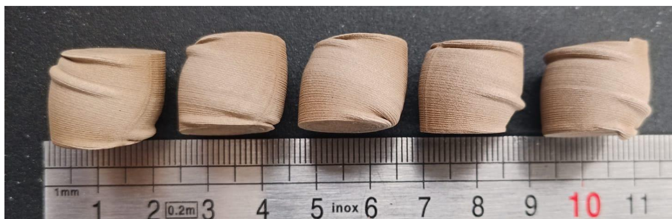
Figure 5. Vertically layered printed samples after compression load.
