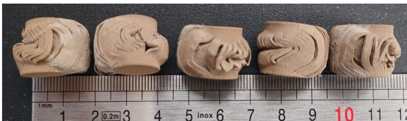
Figure 6. Horizontally layered printed samples after compression load.
