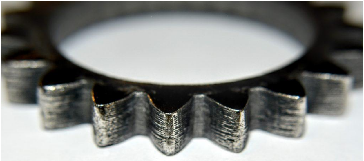
Filamet™ Pure Stainless 316L printed with an Anet A8 (a sub $500, FFF 3d printer)
