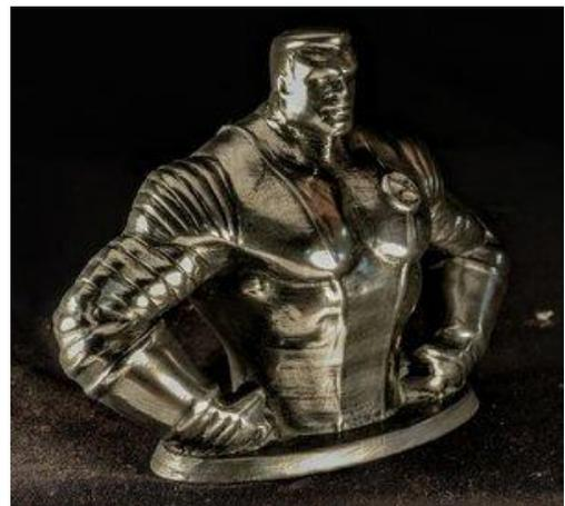
While prints made with Filamet™ can be polished to a beautiful shine in their green state, many applications dictate post-processing. Filamet™ again surpasses other metal AM solutions by debinding with simple heat – no catalysts, no solvents, no safety risk.
