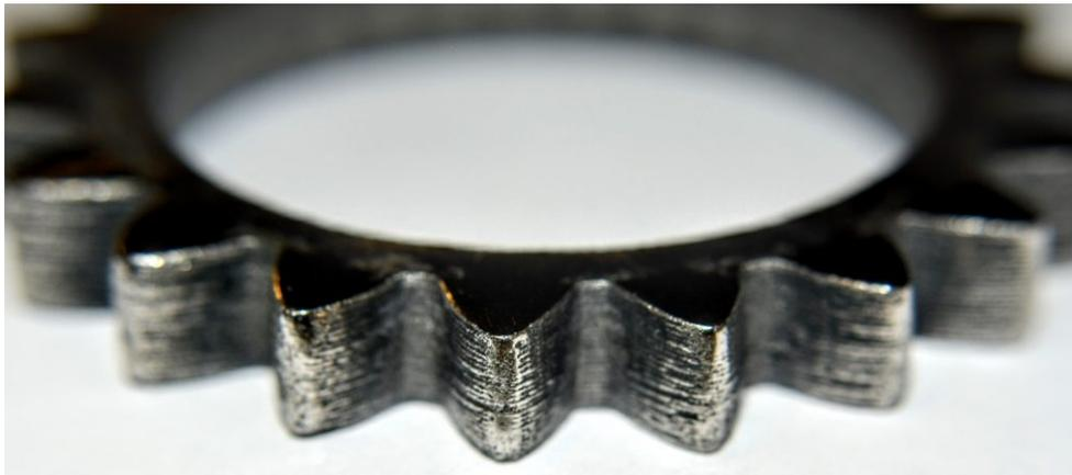
A gear 3D printed
