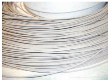
Metal Filamet like the stainless steel 316L can be used with any FFF/FDM 3D printer.
