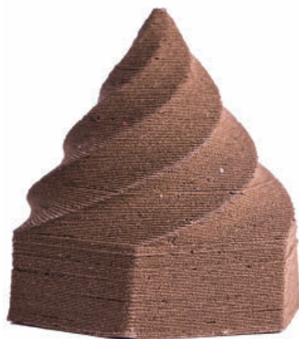
Anet A8 printer builds a bronze swirly cone.
