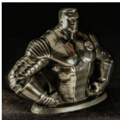
Unsintered filament like the stainless steel used for "Colossus" and copper for the "Thinking Man" can achieve a near mirror finish.
