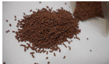
Copper Filamet pellets are used in large-format printers that employ a cone-shaped hopper to funnel the material to the printing bed.
