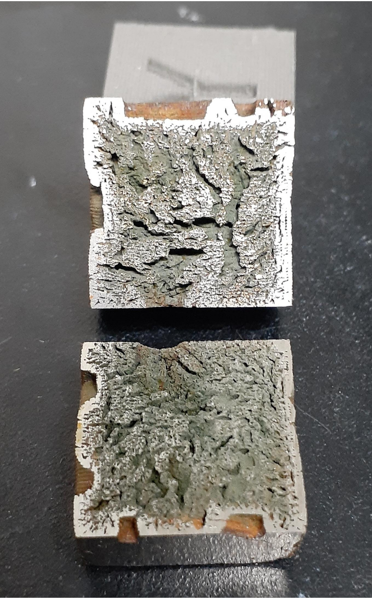
Above is a cutaway of one of the cubes from the first sintering run after the process was complete. Though there is a thin layer of sintered steel visible on the outside edge around the cube, it is clear the process isn't complete. Longer holds and more heat should contribute to more consistent densification, alongside object shrinkage.
