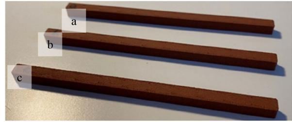
**Fig. 14** Cuboids ( $5.5 \cdot 100 \text{ m}^3$ ) printed with parameter set FB2: **a** CubFB2a, **b** CubFB2b, and **c** CubFB2c
