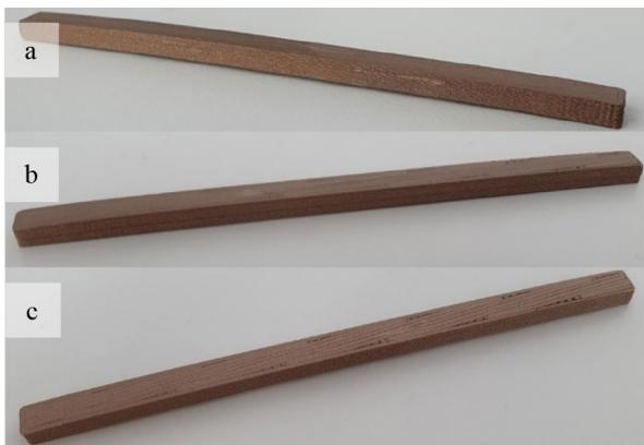
**Fig. 13** Cuboids ( $5.5 \cdot 100 \text{ m}^3$ ) printed with process parameter FA4: **a** CubFAa, **b** CubFAB, and **c** CubFAc
