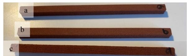
**Fig. 15** Cuboids ( $5.5 \cdot 100 \text{ m}^3$ ) printed with parameter set FB4: **a** CubFB4a, **b** CubFB4b, and **c** CubFB4c
