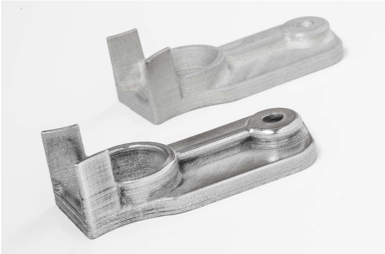
Figure 4: Before (top) and after (bottom) buffing post-processing
