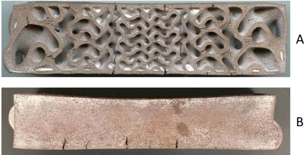
Figure 4.7 Heat exchanger (Model: EXCH 2 TW) Exhibiting Fractures Propagating on Saddle Points, Fabricated through MFDM with printing parameters: 0.21mm Layer Thickness, 100% Extrusion Ratio, 1.2mm Minimum Wall Thickness: A) Top View, B) Side View.
