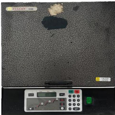
Figure 3.3 Ney Vulcan 3-550 Programmable Furnace Model (Internal Dimensions: 230x230x180mm (WxDxH)).
