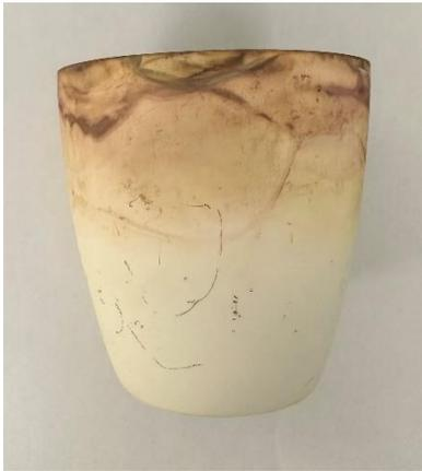
Figure 3.4 300mL Alumina Crucible.
