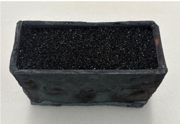
Figure 3.6 Steel Crucible with Granulated Carbon.
