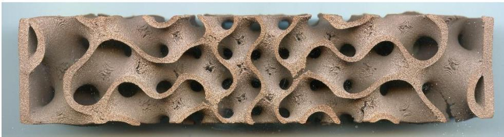
Figure 4.8 Heat exchanger (Model: EXCH RDC) Exhibiting Large Pinholes and Fractures, Fabricated through MFDM Sintering Parameters: Alumina Refractory Ballast, Refractory Plate Thickness 13mm, Sintering Temperature 1074°C, Hold Time 6.5hr, cooling rate 1°C/min: A) Top View, B) Side View.
