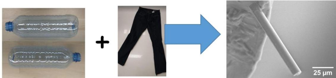
**Figure 1.15 Combining waste products from two streams, plastic food packaging and textiles to create an advanced FFF-compatible composite. Data from [51, 52].**
