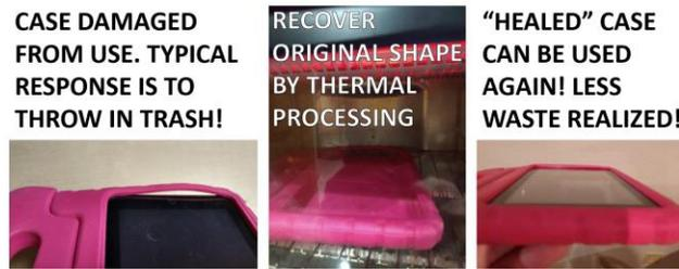
**Fig. 2.2. Using the inherent shape memory properties of EVA to reuse a tablet case.**
