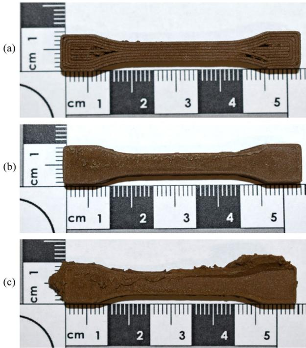
**Fig. 6** Specimens presenting printability issues corresponding to set A (a), set H (b), and set I (c)
