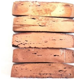
Fig 4: A cross-section of a successfully debound and sintered part.
