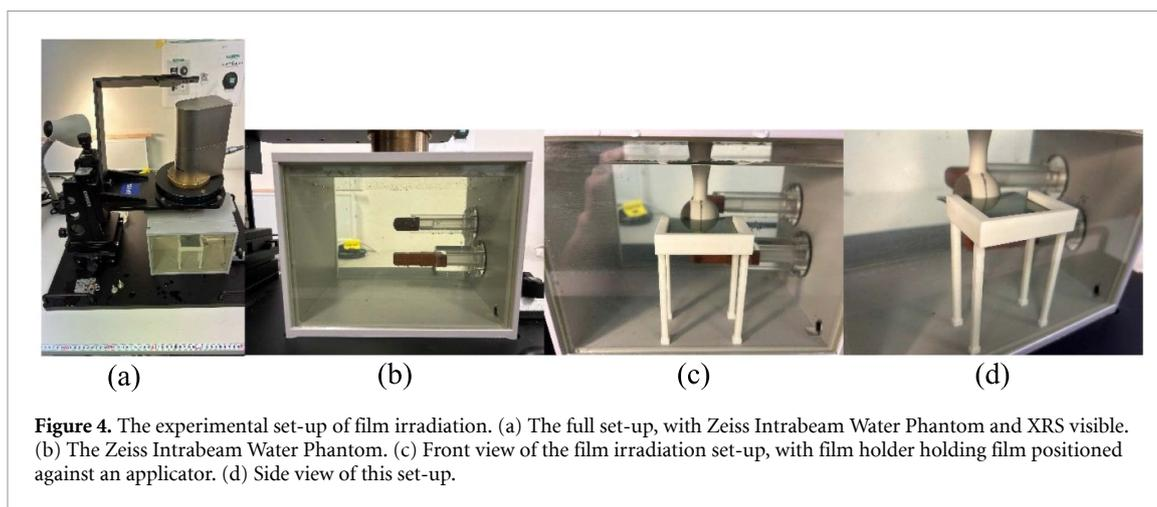
**Figure 4.** The experimental set-up of film irradiation. (a) The full set-up, with Zeiss Intrabeam Water Phantom and XRS visible. (b) The Zeiss Intrabeam Water Phantom. (c) Front view of the film irradiation set-up, with film holder holding film positioned against an applicator. (d) Side view of this set-up.
